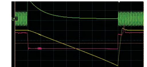
Green color is input voltage Yellow color is output frequency Red color is bus voltage
