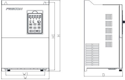
Fig.1-10 22~110kW Wall mounting diagram
