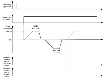
Figure 3.3 Light load direction search timing diagram
