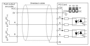
Fig. C-6 Connection schematic diagram of EXC-PG01
