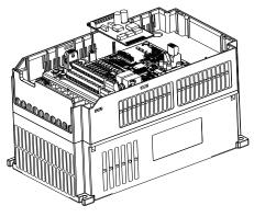
Fig.C-1 PG card installation
