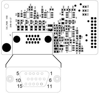
Fig.C-9 EXC-PG06 Sin-Cos encoder PG card
