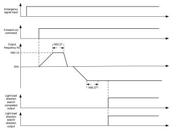
Figure 3.4 Light load direction search timing diagram
