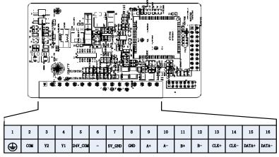
Fig.C-8 EXC-PG05 ECN1313 PG terminals
