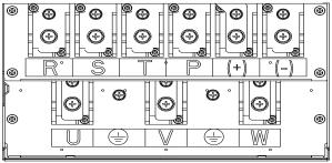
Fig.1-7. 90~110kW Main Circuit Terminal Diagram
