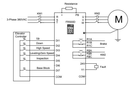
Fig. 2-2 Wiring of two multi-step speed terminal elevator controller
