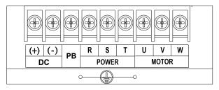
Fig.1-5. 22~37kW Main Circuit Terminal Diagram
