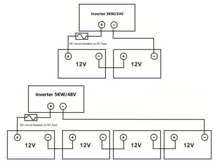
5. Insert the battery wires flatly into battery connectors of inverter and make sure the bolts are tightened with torque of 2 Nm in clockwise direction. Make sure polarity at both the battery and the inverter/charge is correctly connected and conductors are tightly screwed into the battery terminals. Recommended tool: #2 Pozi Screwdriver
