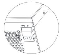
4. Check correct polarity of wire connection from PV modules and PV input connectors. Then, connect positive pole (+) of connection wire to positive pole (+) of PV input connector. Connect negative pole (-) of connection wire to negative pole (-) of PV input connector. Screw two wires tightly in clockwise direction. Recommended tool: 4mm blade screwdriver
