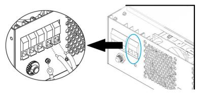
5. Make sure the wires are securely connected.
