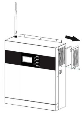
Step 3: Clean air filter foam and dustproof case. After clearance, re-assemble the dust-kit back to the inverter.
